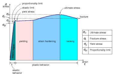
Brittle materials, like glass, have  $\sigma_u \approx \sigma_y$ . Unlike the elastic modulus, the yield stress can vary greatly from one alloy to the other. Spring steel wants to have a very high yield stress, for instance. Here are some numbers:
