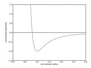
The figure shows the form of the potential when m=6 and n=3. This is in the empirical range for many crystalline bonds. Ionic bonds may have n=1. It is traditional to have m=2n, though I don't know how well-motivated this choice is. Van der Waals potentials are better described with m=12 and n=6. If we demand that the potential has a minimum at r=a and  $V(a)=-\varepsilon$ , then we get:
